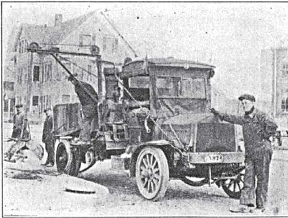
STANDARD MOTOR TRUCK EQUIPPED FOR CLEANING SEWER CATCH BASINS, PAWTUCKET, R. I.
