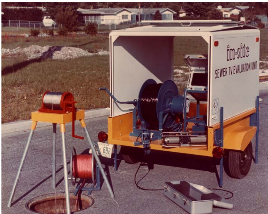
Figure 10. Hand winch skid mounted camera Source: Cues archival history
