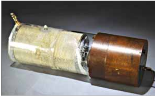
Figure 4. The 1927 version of Farnsworth's image dissector. He received a patent for the image dissector in 1930, and successfully defended that patent against Vladimir Zworykin and David Sarnoff. Courtesy: Smithsonian Institution. Source: http://www.ieee-virtual-museum.org/collection
